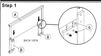
Fix head bottom leg left & right tio the head board top with minifix '6' as shown.
