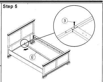
Fix center bar 'E' to the cross bar 'F' with bolts '3' as shown.
