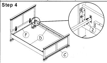
Fix cross bar 'F' to the side rail with bolts '2' as shown.
